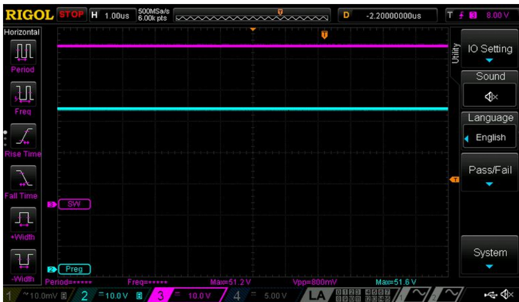
Fig. 10: Pre-regulator in 100% duty cycle, without load connected
