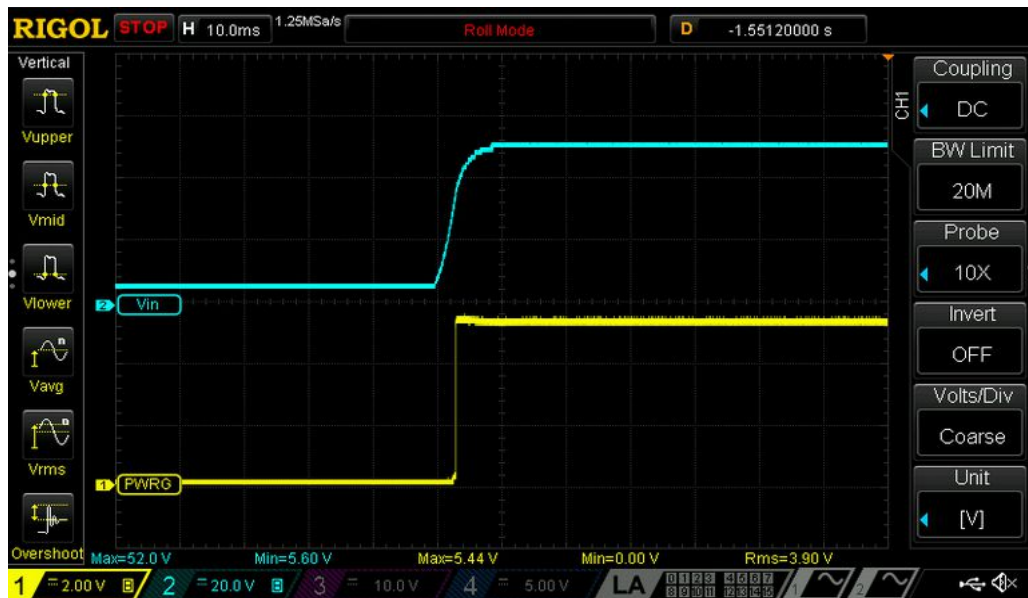
Fig. 11: PWRGOOD signal transition (Power on)
