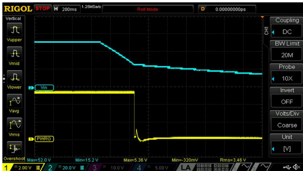
Fig. 12: PWRGOOD signal transition (Power off)
