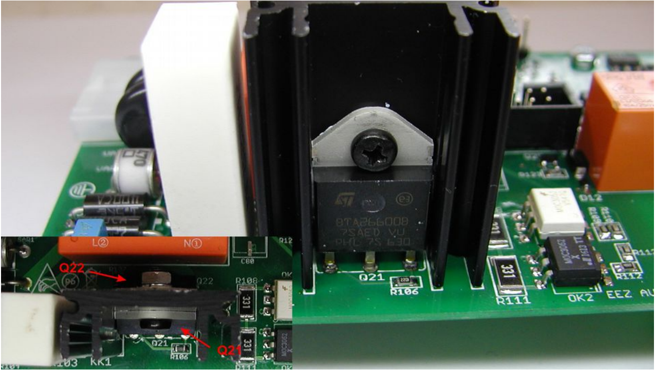
Fig. 2: Q21 and Q22 shares the same heatsink (KK1)
