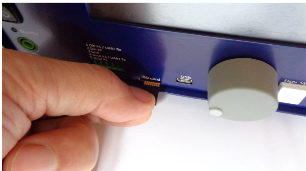
Fig. 5: Micro SD card insertion
