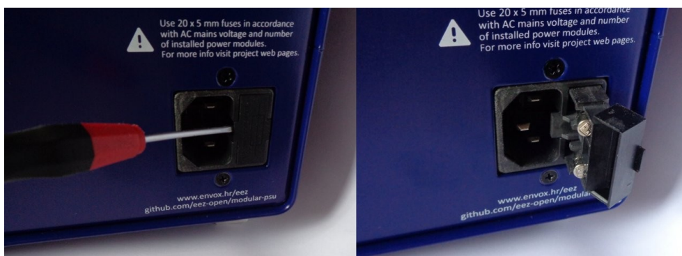
Fig. 2: Opening the fuse holder
