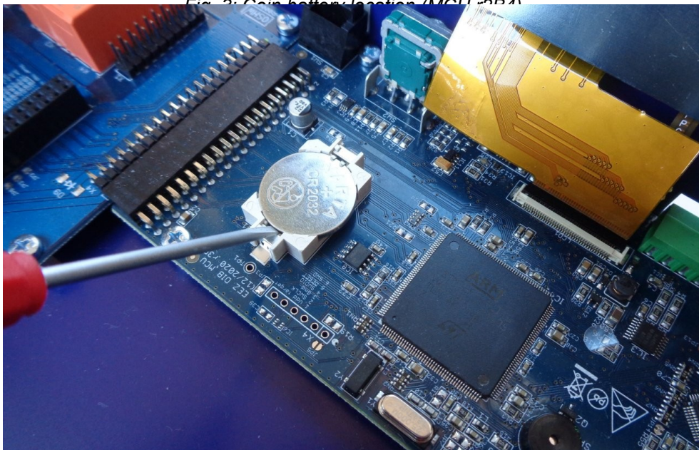
Fig. 4: Coin battery location (MCU r3B3)
