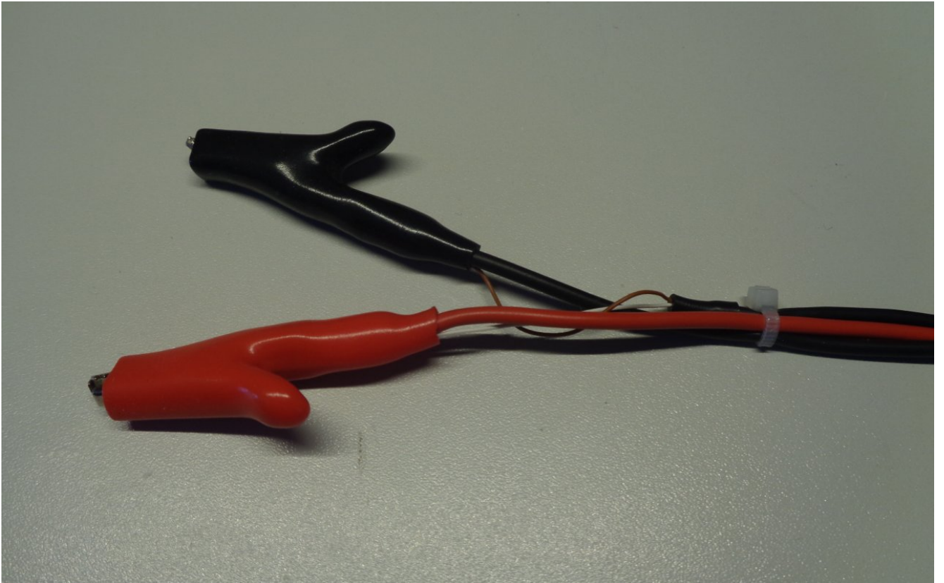
Fig. 6: 4-wire (Kelvin) clip for remote sensing
