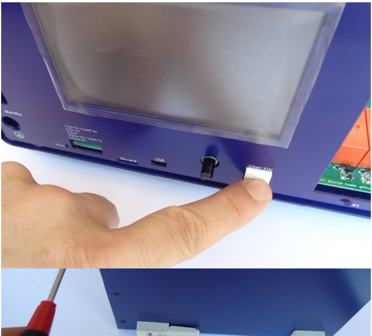
Fig. 16: Fixing the front panel from below to the bottom plate
