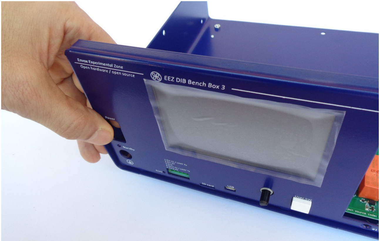
Fig. 14: Checking that the encoder shaft and user switch are in place
