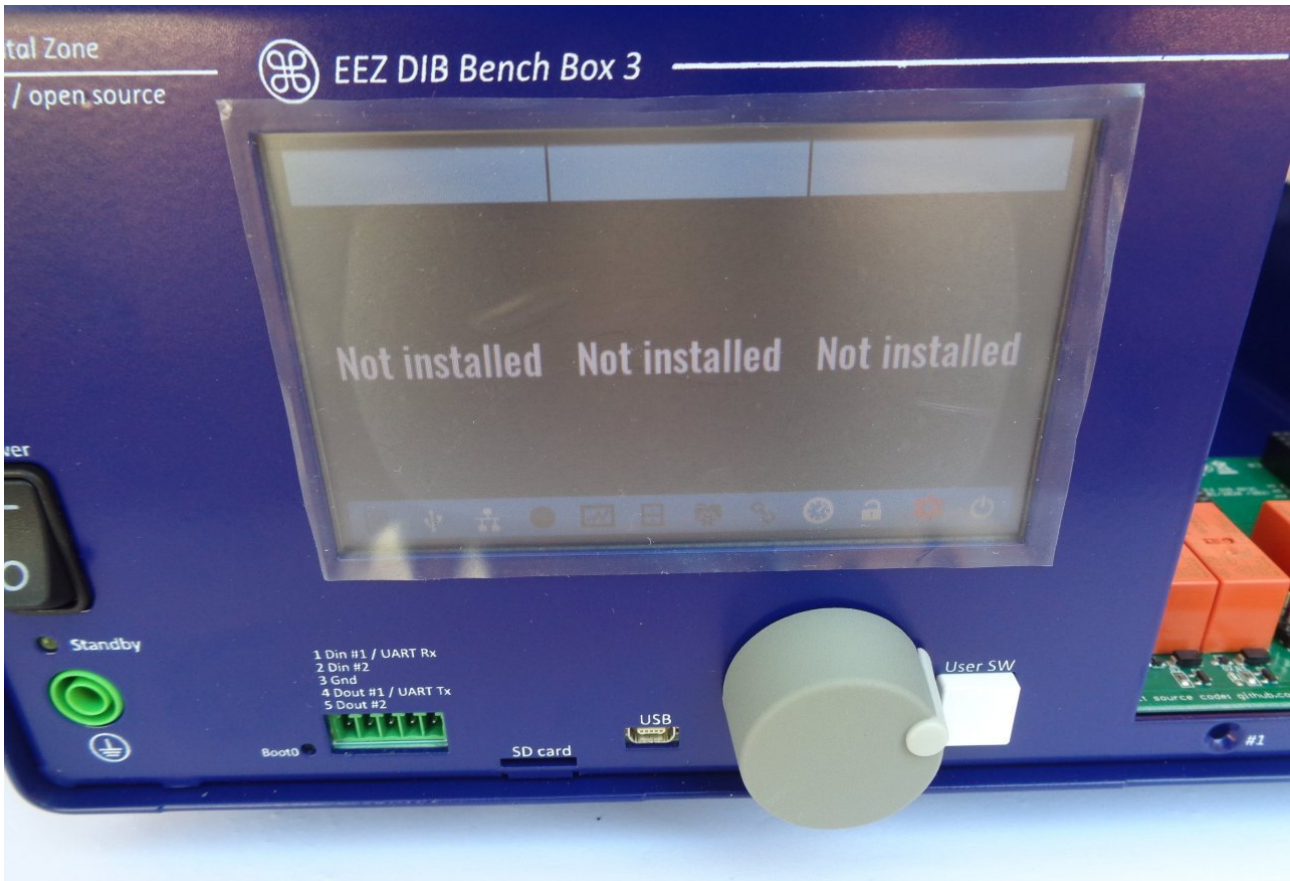
Fig. 29: Test power up without peripheral modules or micro SD card
