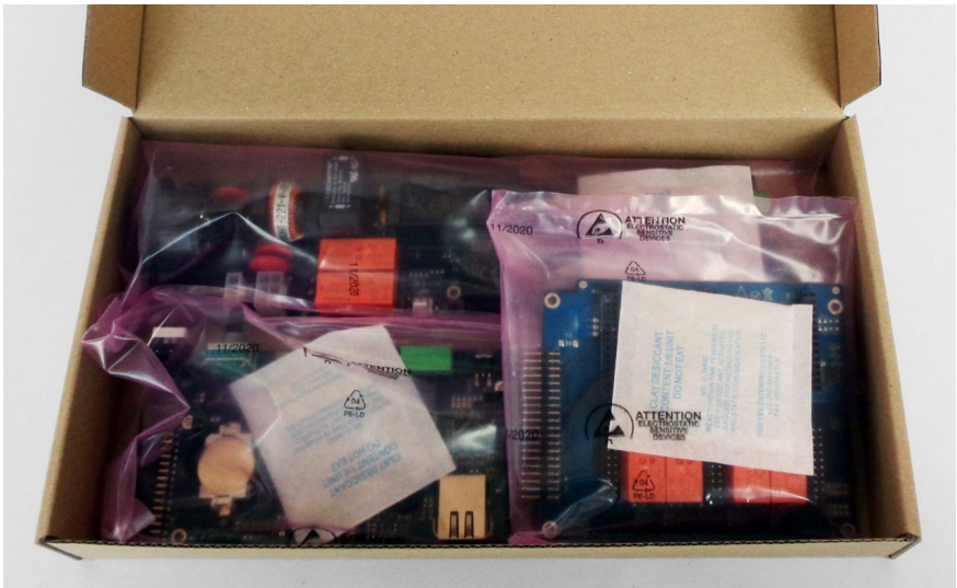
Fig. 3: r3B3 base modules (SD card is already installed on the MCU module)
