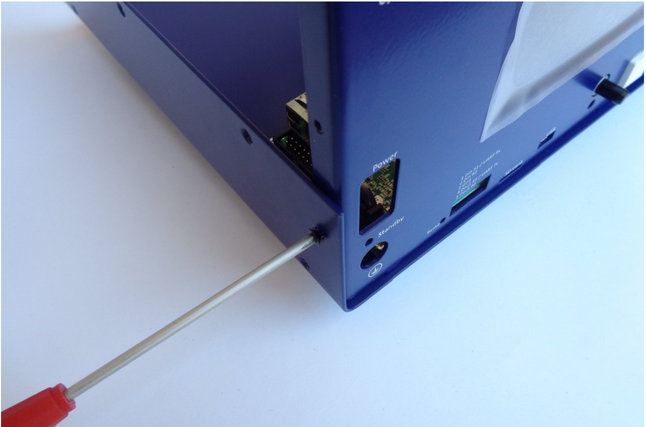
Fig. 17: Fixing the front panel from the side to the bottom plate
