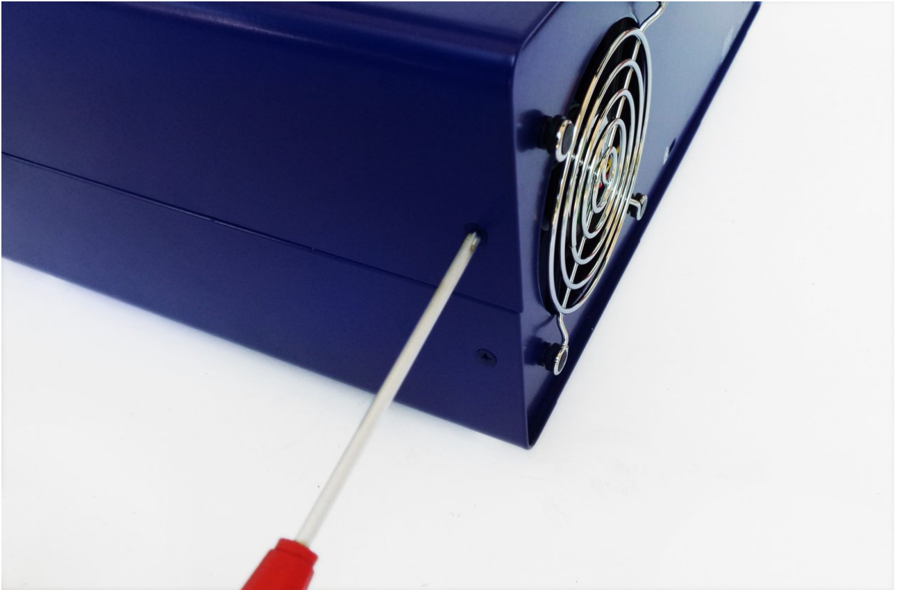
Fig. 42: Securing the top cover
