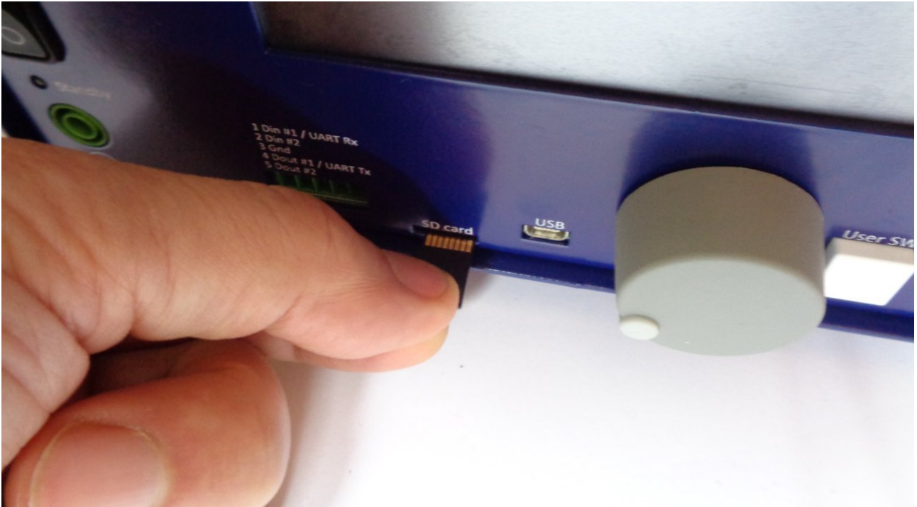
Fig. 30: Inserting micro SD card
