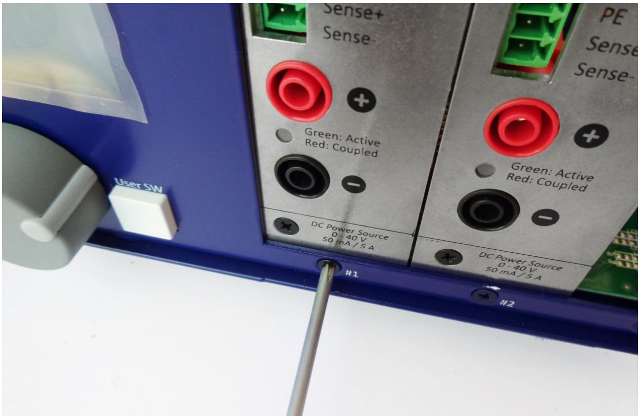
Fig. 40: Power module fastening
